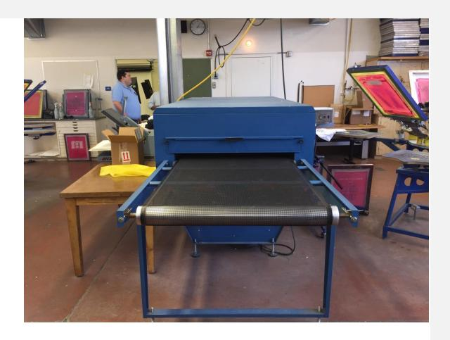
Loading end of the conveyer drier for heat curing printed shirts
